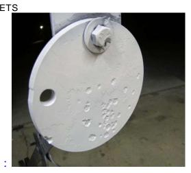
• Flat metallic targets must be set parallel to the firing line. Note: Metallic targets that are not parallel to the firing line will produce a unsafe side ricochet zone from the target face that could cause splatter to adjacent shooters. (See Diagram)
